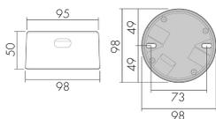
Abmessungen in mm
