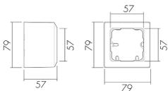
Abmessungen in mm
