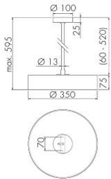
Abmessungen in mm
